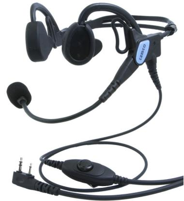
Bone conduction headset HG21 is equipped with high output bone vibration speaker. In ordinary environment, ambient sound is audible with the headset mounted since both ears are not covered. Under deafening noise, combined use of the anti-noise ear plugs enables clear transmission because bone conduction speaker transmits incoming voice directly to the auditory nerve.
